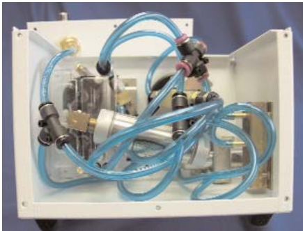
Clippard's R-331 timing valve, behind the tubing.
